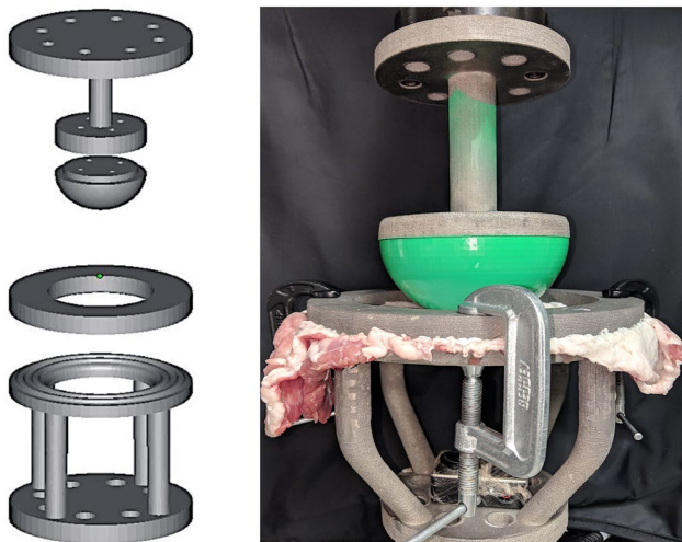
Fig. 2 Ball-burst Apparatus—Right—3D printed titanium with plastic head colored green. Upper portion includes spherical head attached to piston in order to apply force to the sample being held in the ring below. Left: computer-aided design (CAD) image of ball-burst apparatus. Ring diameter of ball-burst apparatus is 7 cm (color figure online)
